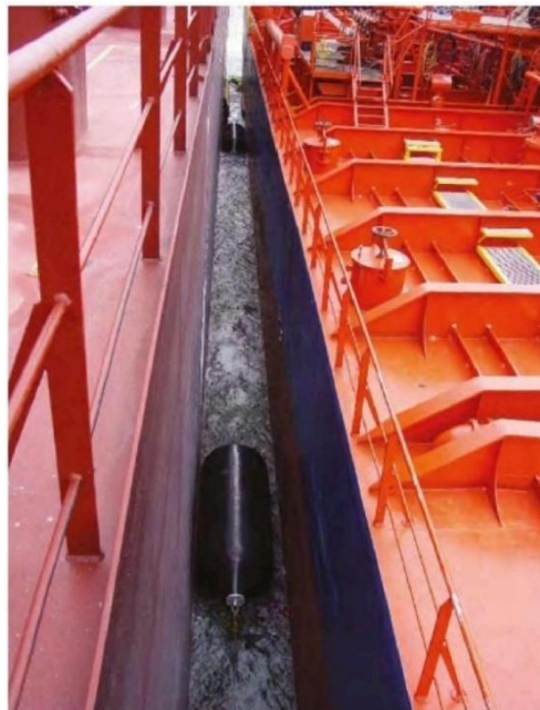
Figure 4.1.5 Foam fenders in use for an in port transfer
