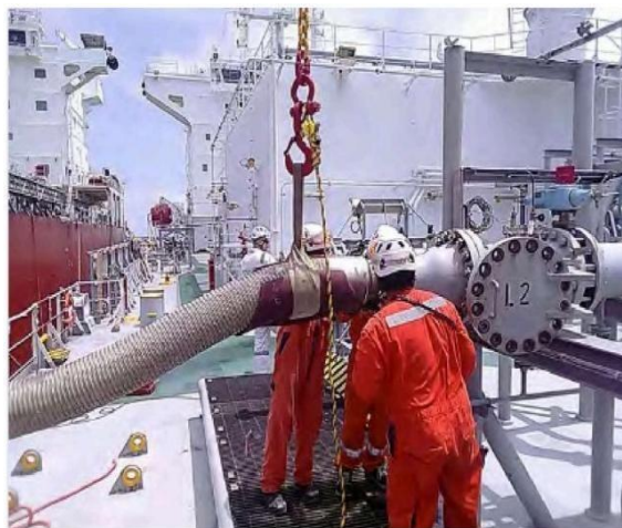
Figure 8.1.2 Hose connection on LPG STS operation
